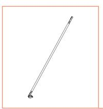
Used for stiffening the scaffolding. Made of pipe 42 mm in diameter fitted with rotary clamp. Installed by slinging the upper end of the bracing into the gusset opening of vertical frame and fixing the other end to the bottom of opposite vertical frame using the clamp.
