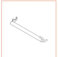
Installed in cut outs in frame gusset plates using one standard coupling, enabling free adjustment of distance between scaffolding and the wall and transferring external load from scaffolding to the building.
