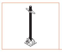
Tiltable threaded pipe connector on 150 x 150 mm base, fitted with a nut and a clamp for pipe the diameter of 48.3 mm. Used for setting up the frame on inclined surfaces.
