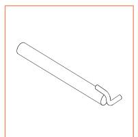
Long anchoring connectors (length of 1.30 m and 1.50 m) are fixed to both stands of vertical frames using two standard couplings. Short anchoring connectors (length of 0.40 m and 0.80 m) are fixed to just one frame stand, located near the wall, using one standard coupling.
