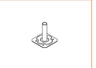
150 x 150 mm base jack with pipe stud diameter of 36 mm, for correct setting of scaffolding that does not require height adjustment.
