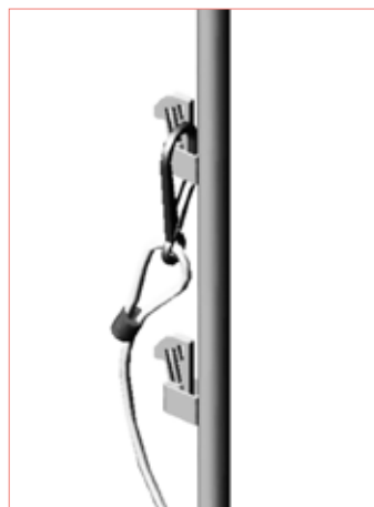
Fig. 2.2a – Attachment to the wedge cartridge
