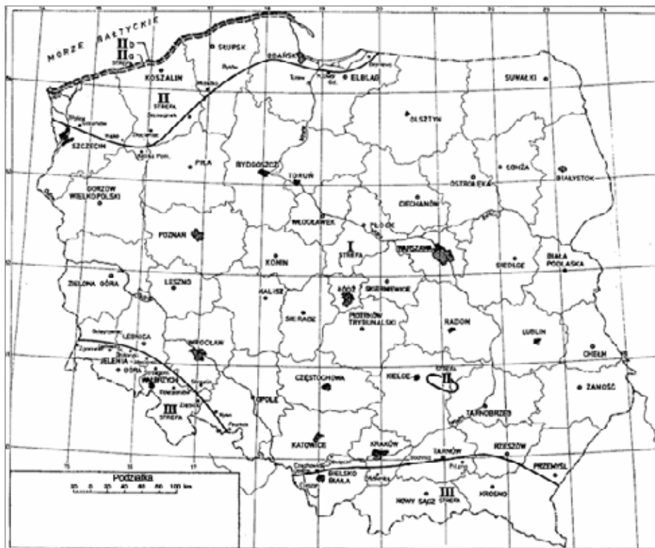
Fig. 4.1 – Wind load map according to PN-77/B-02011
